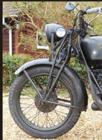
Below: here we see the front girder forks with its three coil springs.
